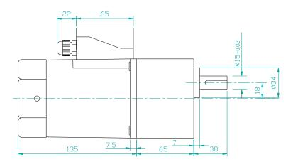
Motor Round Shaft with Terminal Box
