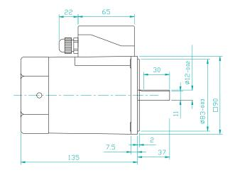
Motor, Gearbox with Lead Wires
